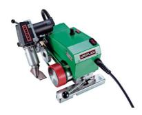
To thermally weld a waterproof seal between two sheets of BENFELT:
