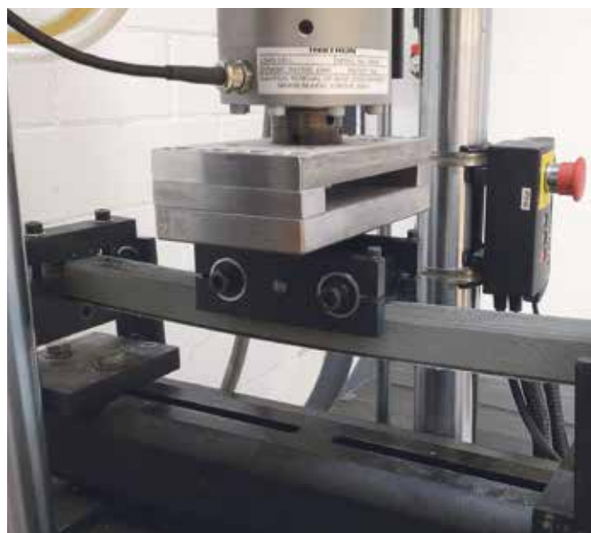
Fig. 13: Dynamic test on sandwich panels with RAVATHERM™ XPS X core
