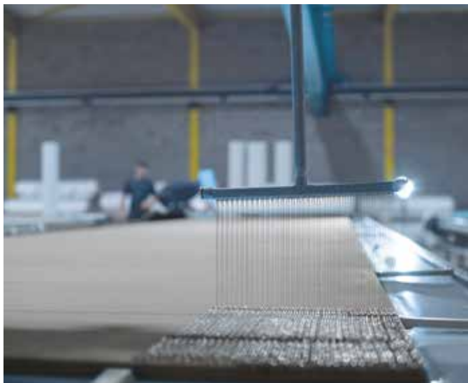
Fig. 16: Application of a 2 component PU adhesive
