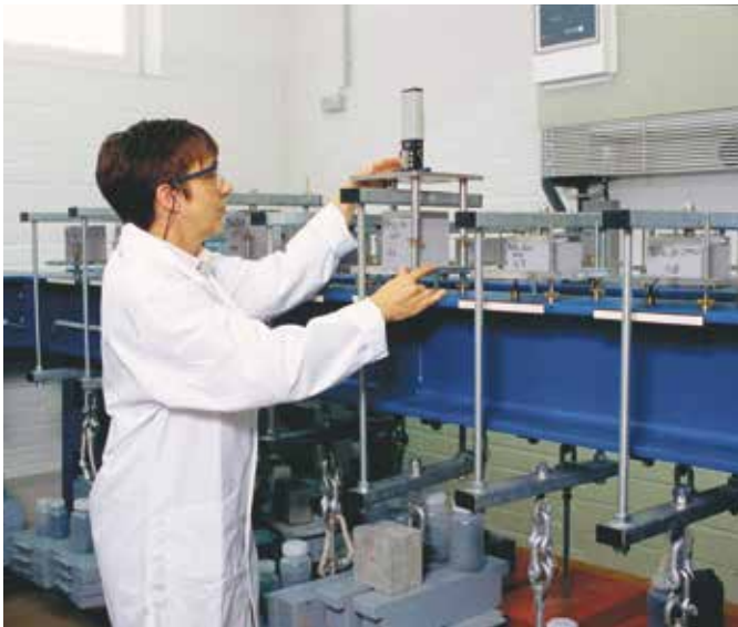
Fig. 11: Testing creep performance in Ravago's dedicated laboratory
