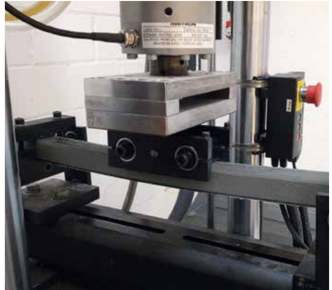
Fig. 13: Dynamic test on sandwich panels with RAVATHERM™ XPS X core
