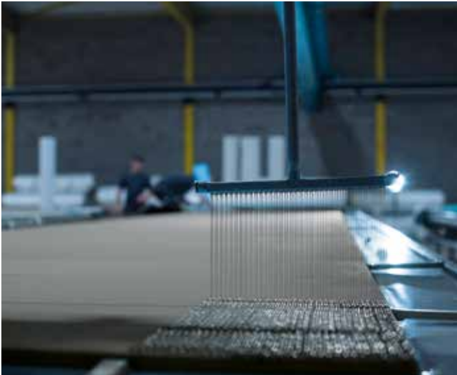
Fig. 16: Application of a 2 component PU adhesive
