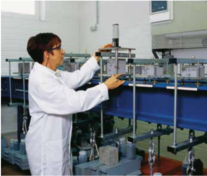
Fig. 11: Testing creep performance in Ravago's dedicated laboratory
