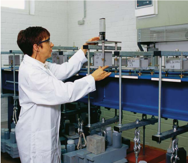
Fig. 07: Testing creep performance in Ravago's dedicated laboratory
