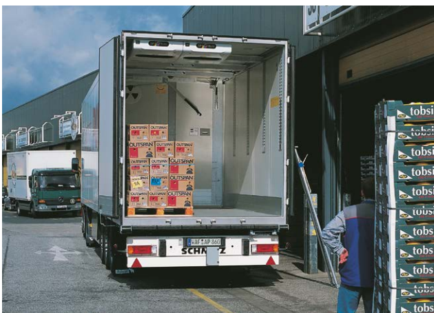
Fig. 09: Well insulated and able to support loads: refrigerated truck bodies using RAVATHERM™ XPS core panels.
