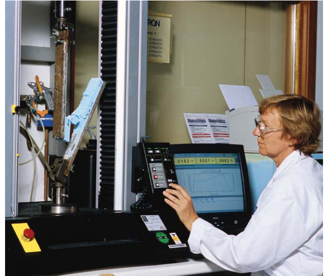
Fig. 08: Shear test in Ravago's dedicated laboratory
