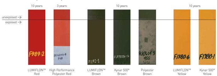
ALPOLIC<sup>TM</sup> Paint Coating is usually evaluated with chamber tests such as accelerated weathering test, salt spray etc., but it is also checked regularly by means of actual exposures over decades in the harsh climate coastal areas (Numazu, Japan and Florida, USA).
